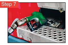
Activate the nozzle by engaging lever on dispenser. Then pull trigger and begin dispensing fuel.
